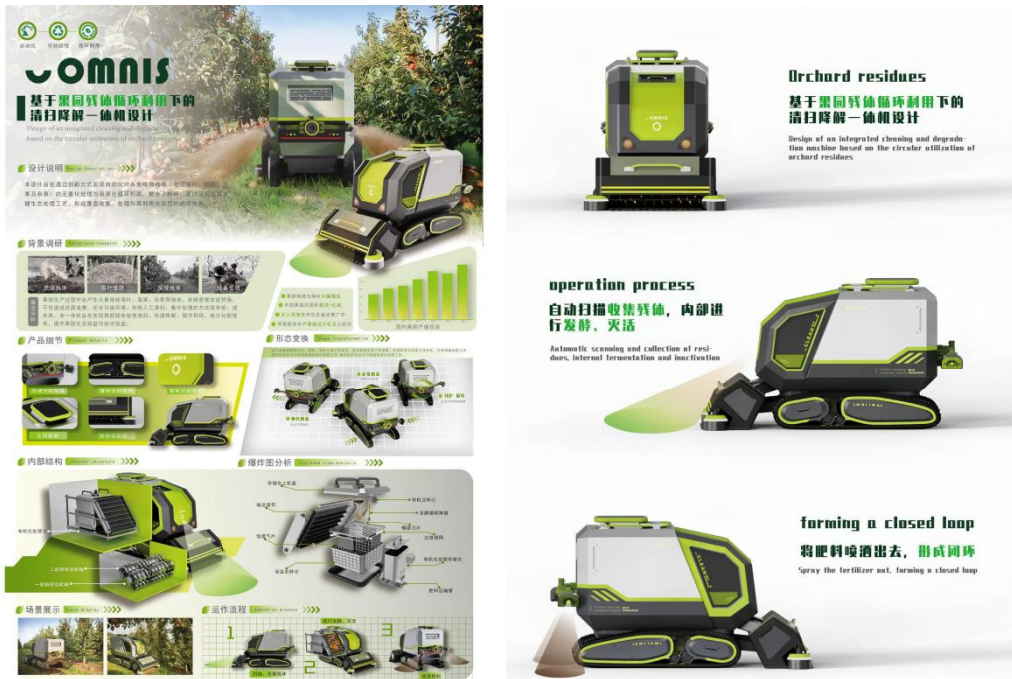
Figure 7-1 and 7-2 Design of a Sweeping and Degrading Integrated Machine for Orchard Residue Recycling
